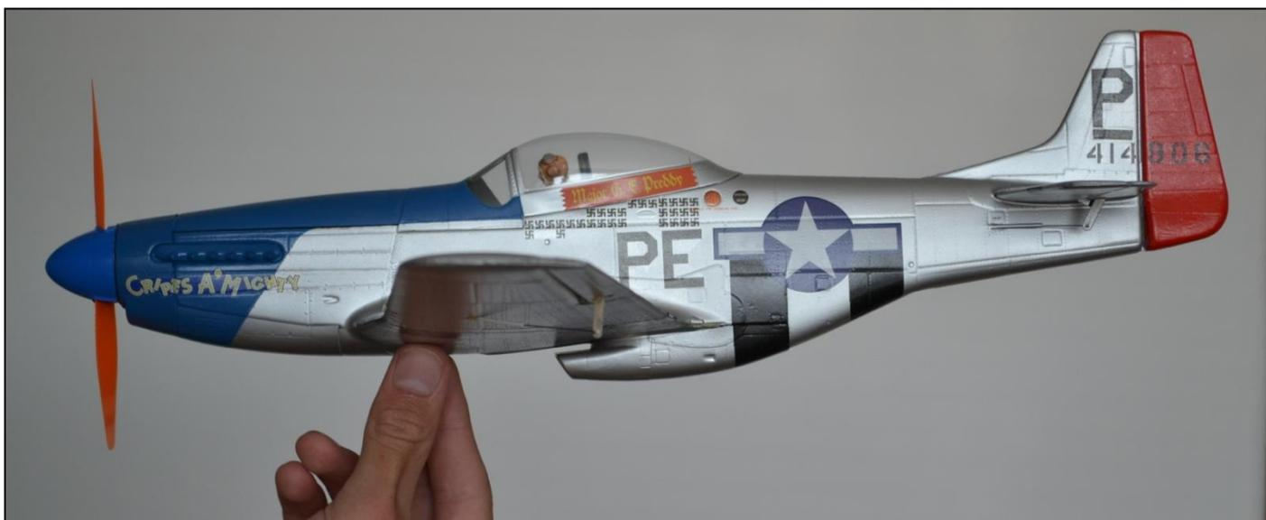
The wing could be made either detachable, or glued to the fuselage. In order to save weight and provide for more rigidity to the model we suggest tack-gluing (PU, UHU Por) the wing to the fuselage. Still, if need be, the glue tacks could be carefully cut through and the wing removed again.
