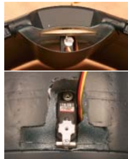
By recessing the aileron servo through the center section of the wing I was able to minimize any binding in the pushrods. The basswood servo rails are glued to the bottom of the wing center section. The fuselage belly pan protects the servo from landing damage.
