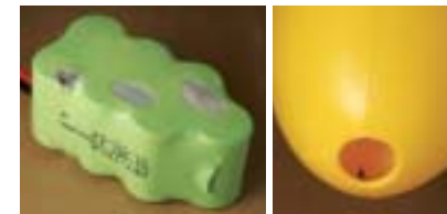
Without cooling airflow, my battery got hot enough to melt the heat shrink covering. Drilling a dime-size hole in the nose of the fuselage provides all the necessary cooling.
