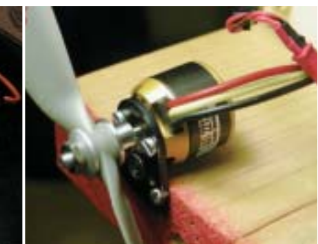
Left: The author with the 2212/26 on a test stand. Center: The test setup, including the Astro Flight servo tester and Micro Whattmeter, a Jeti 18-3P controller, and my trusty old NorCal Avionics Accu-Tach 1. Right: Close-up of the motor mount for testing the little AXIs—one frame from a Maxx Products Speed 400 gearbox.
