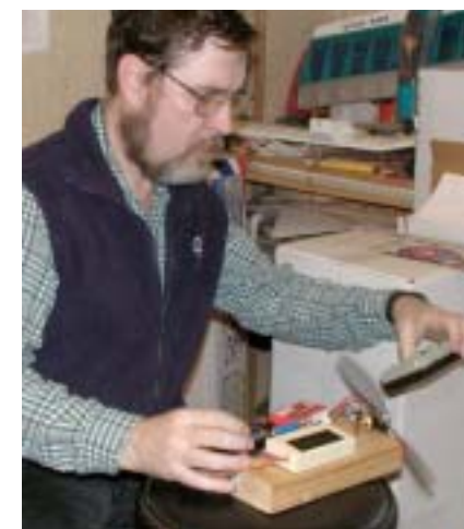
Left: The author with the 2212/26 on a test stand. Center: The test setup, including the Astro Flight servo tester and Micro Whattmeter, a Jeti 18-3P controller, and my trusty old NorCal Avionics Accu-Tach 1. Right: Close-up of the motor mount for testing the little AXIs—one frame from a Maxx Products Speed 400 gearbox.
