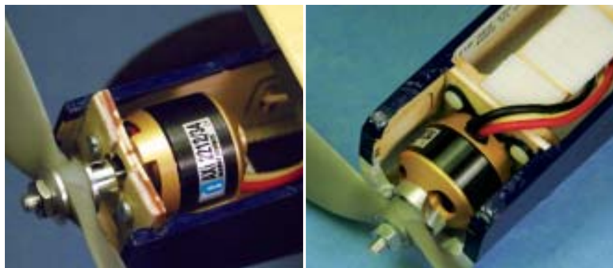
Left: AXI 2212/34 mounted from the front in the Electroflying Models eSKA. Right: AXI 2208/34 in the CI-i-max Models Sin-Naps, using the rear mount kit.
