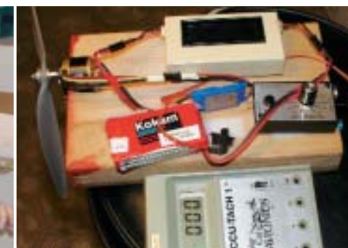
Left: The author with the 2212/26 on a test stand. Center: The test setup, including the Astro Flight servo tester and Micro Whattmeter, a Jeti 18-3P controller, and my trusty old NorCal Avionics Accu-Tach 1. Right: Close-up of the motor mount for testing the little AXIs—one frame from a Maxx Products Speed 400 gearbox.
