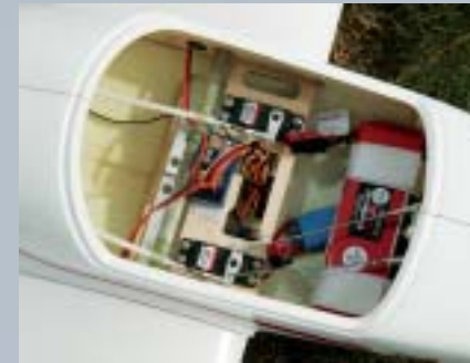
The lower servo controls both the rudder and the nosewheel; the upper servo actuates the elevator. Note the ample room in the fuse.
